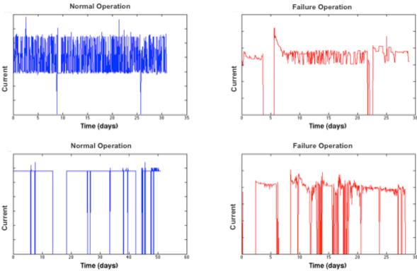
Figure 4: Examples of current measurements during normal operation (blue) and failed operation (red).
