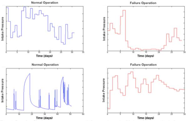
Figure 3: Examples of intake pressure measurements during normal operation (blue) and failed operation (red).
