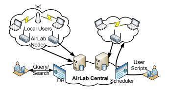
Figure 1: AirLab Architecture. AirLab includes measurement nodes located at member sites that perform local measurements and send traces back to AirLab Central. Users can query the collected data, as well as schedule customized measurement tasks written as scripts calling AirLab's measurement API.
