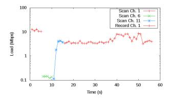
Figure 2: Baseline experiment visualization. The node scans active channels 1, 6 and 11 and picks the highest utilized channel 11 for recording baseline data.
