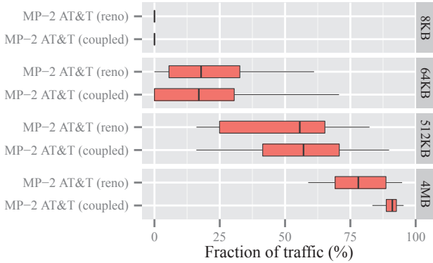
Figure 7: Amherst coffee shop: fraction of traffic carried by the cellular path. With MPTCP-coupled and uncoupled New Reno TCPs, where MPTCP is in favor of the cellular path when the file size increases.
