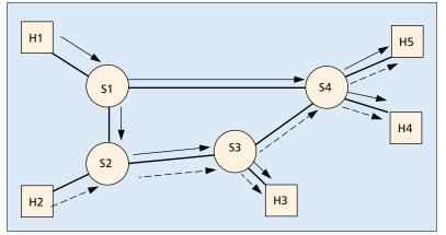
**FIGURE 1.** A simple network topology with the multicast routing trees. H1 and H2 are data sources, and H3, H4, and H5 are receivers. The solid lines depict the routing tree of H1; the dotted lines depict the routing tree of H2. In general, the set of sources and the set of receivers may overlap partially or completely. For the sake of clarity, here they are disjoint.
