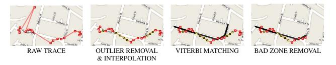
Figure 6: The Map Matching process. A raw location trace is gradually refined to produce a final, high quality street route. In this example, due to noise and outages, only the first three segments produced quality estimates.
