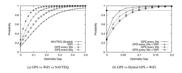
Figure 8: CDF of Optimality Gap when route planning using VTrack. Larger optimality gaps are worse.
