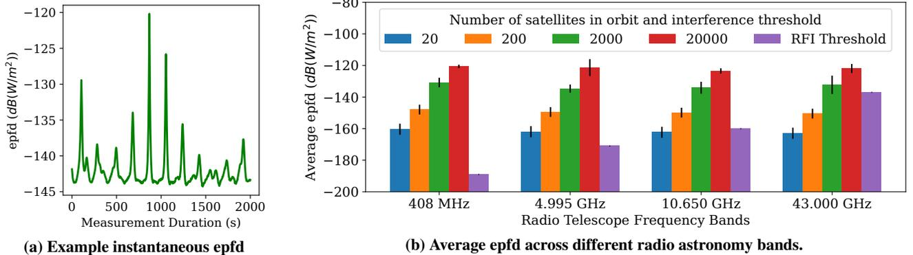
**Figure 3: Equivalent power flux density (epfd) is a measure of the total power emitted by a group of satellites per unit area, normalized to a reference frequency and bandwidth, expressing the combined effect of their transmissions on radio astronomy observations. (a) epfd during a 2000-second measurement for 2000 satellites. (b) Average epfd for different number of satellites and frequency bands. The error bars show the standard deviation of 24 runs of the simulator.**
