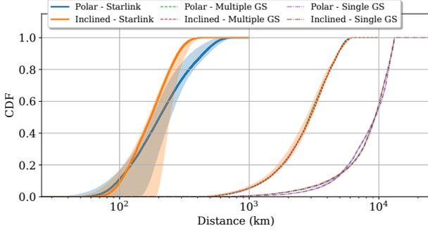
**Figure 4: CDF of the distance from 500 LEO satellites to the nearest Starlink satellite or ground station(s). The center line is median CDF value, and shaded areas cover the 10% to 90% values.**
