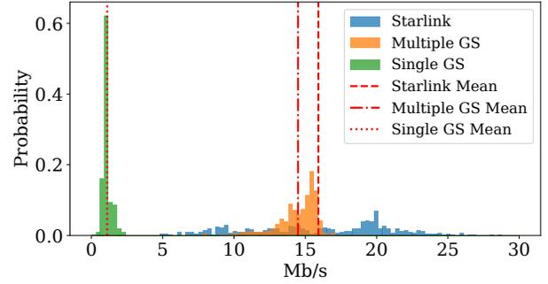
**Figure 5: Average upload throughput over 24 hours under different connectivity models, simulated for 500 LEO satellite orbits. The mean throughputs are 15.9, 14.5 and 1.1 Mbps for Starlink, multiple and single ground stations.**
