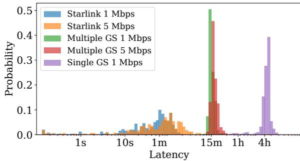
**Figure 6: Satellite upload latency under different connectivity models, simulated for 500 LEO satellite orbits and 1 and 5 Mbps constant traffic demand.**
