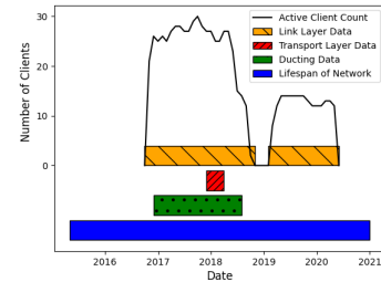
Figure 3: Timeline of the network and our datasets. The client count is based on our link layer data. The period in 2019 with 0 clients is therefore due to missing data. We have weather data for the entire lifespan of the network.
