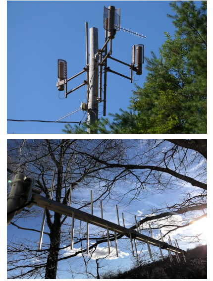
Figure 2: On top, a photo of the antennas for the tri-sector tower (base stations 1-1, 1-2 and 1-3). Below that, a photo of a client antenna.
