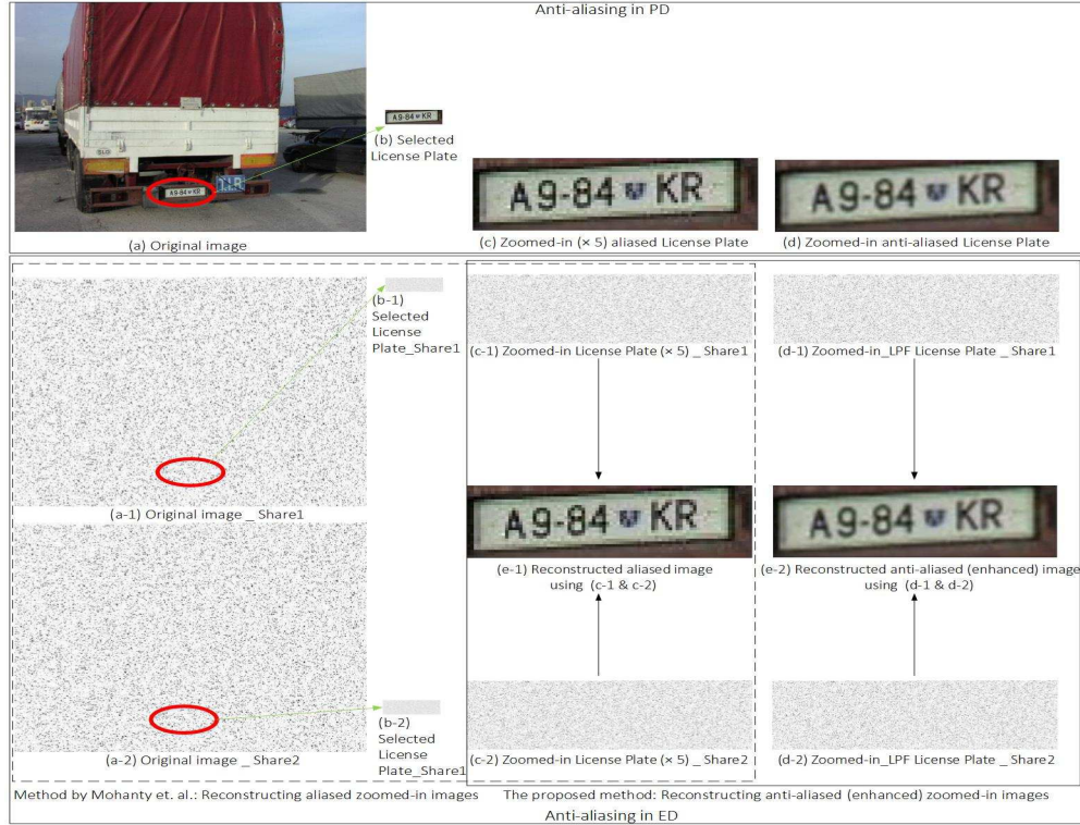
Fig. 6: Depicting the problem of aliasing or checkerboard effect in PD and comparing its removal using proposed Scheme I w.r.t. [Mohanty et al. 2013] in ED
