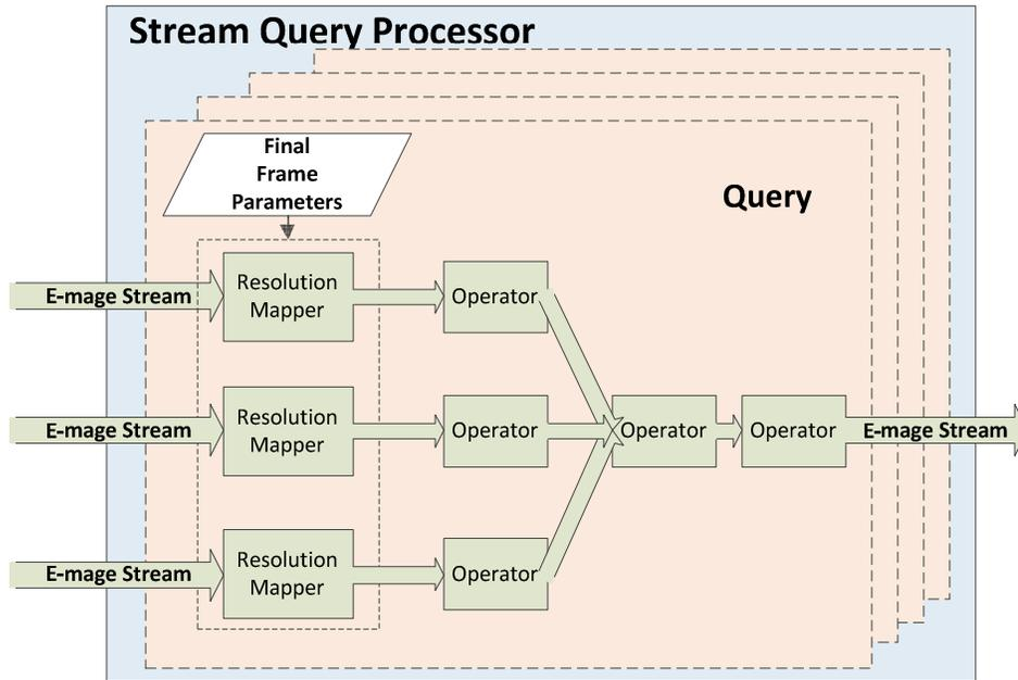
Figure 5. System Architecture of Query Processor
